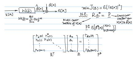
Two perspectives leading to the optimal filter's condition (NE):
