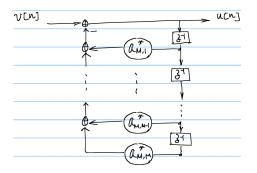
If  $\{v[n]\}$  is a white noise process, the synthesis output  $\{u[n]\}$  using linear prediction is an AR process with parameters  $\{a_{M,k}\}$ .
